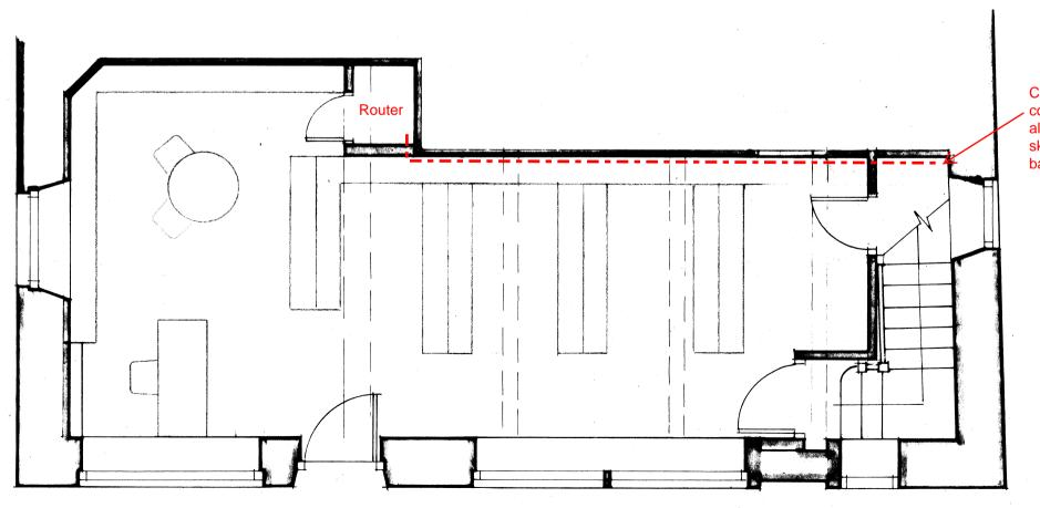
Cable drop down in corner to skirting level along and into end of skirting trunking along back wall of Library.
